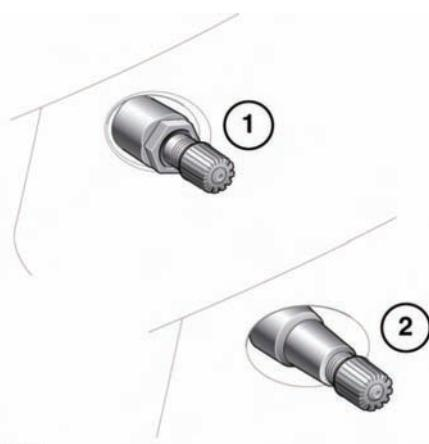
Wheels fitted with a TPM system can be visually identified by the external metal lock nut and valve (1). All Jaguar non-TPM system wheels have a rubber valve fitted (2).
