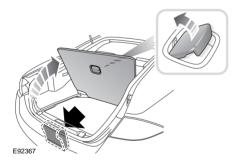
The tyre repair kit is located in the rear underfloor storage compartment.
