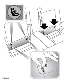
Their location is highlighted by the small tag labels with a child seat graphic. The anchorage loops are located approximately 60 mm (2.5 inches) below each label. Pull back the side of the trim to reveal the aperture and the anchorage loops.
