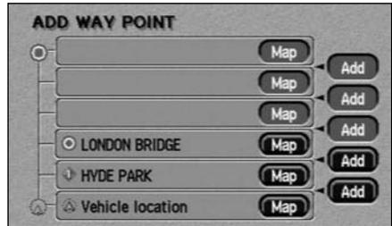
After selecting **Way Pt.** again from the Confirm Destination screen, the Add Way Point screen is displayed. This screen lists the way points already entered, and the destination (if entered).
