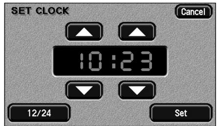
Clock adjustment on S-TYPE and X-TYPE is made by touching the hour or minute up or down arrow button.
