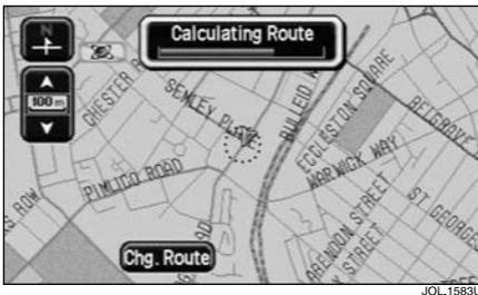
While under guidance, if the vehicle deviates from the route, a new route will be calculated automatically. While the route is being recalculated the screen shows 'Calculating Route' and the time and distance to destination information is replaced by the straight-line distance and direction to the destination.
