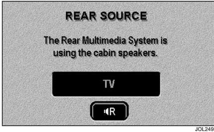
In **REAR MULTIMEDIA** mode, when the rear multimedia system is using one of its own audio sources to play through the cabin speakers in the car, the front screen above is displayed. The possible audio sources from the rear multimedia are, DVD, AUX1, AUX2 (when selected from the rear multimedia system and not from the front).
