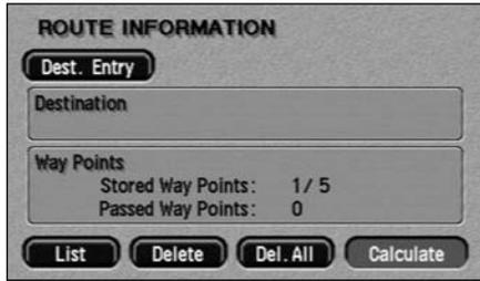
After selecting **Way Pt.** for the first time from the Confirm Destination screen, the address entered is stored as the first way point, and the Route Information screen is displayed, as shown above. This screen also shows details of the destination (if entered).
