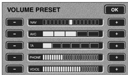
After touching the **Volume** button, the screen displays the buttons for adjustment of volume associated with the navigation system, JaguarVoice, telephone, traffic announcements and automatic volume control (AVC).
