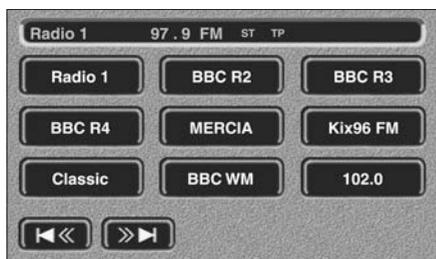
In AM/FM mode, touch-screen buttons provide for station selection and re-tuning. In addition, the upper panel displays waveband, **TA** and **PTY** as selected using the buttons on the radio panel.
