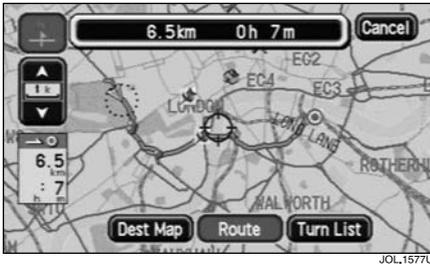
After selecting **Display Whole Route**, the screen shows the whole route, with the total route distance, and estimated travelling time displayed at the top of the screen. Where the route includes a ferry crossing, a ferry icon is shown.
