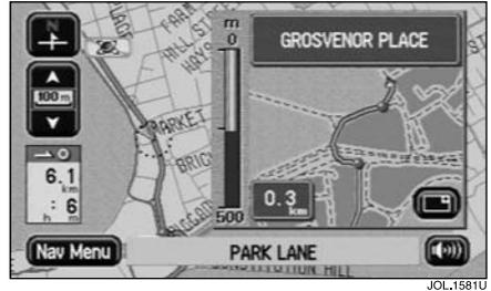
The guidance screen overlay is always displayed while the Split Screen option is selected, and is also displayed when selected manually while the Full Screen option selected.
