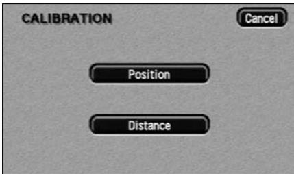
Sometimes the vehicle position may not be correct. This can occur, for example, if the vehicle has been moved on a trailer or by ferry. If the new position is not found automatically by the system, it can be corrected by using the calibration procedures (Position first).
