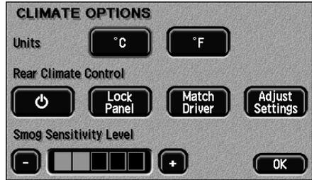
The Options button is displayed in place of the °C/°F button if the optional smog sensor and/or rear climate control panel (4-zone system) are fitted (The XJ only).
