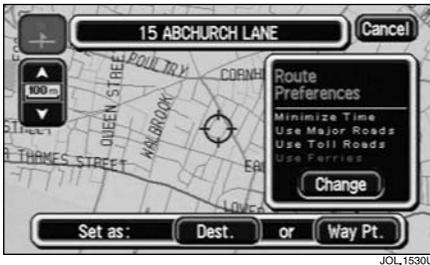
After entering an address, or selecting a map location, the map screen is displayed showing its location. The address details are shown at the top of the screen. The address can be stored as a destination or as a way point.
