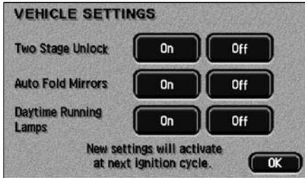
After touching the **Vehicle Settings** button, the screen displays the buttons that switch certain functions on or off.
