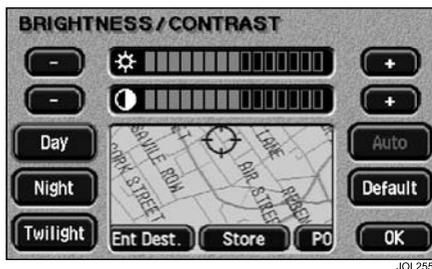
After touching the **Brightness/Contrast** button, the screen displays the buttons for adjustment of the screen display characteristics. The centre window shows the currently selected navigation view.
