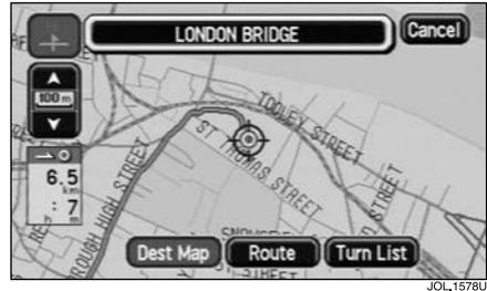
After touching **Dest Map**, the screen shows the last portion of the route, with the destination address displayed at the top of the screen.
