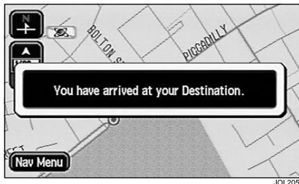
When the vehicle reaches the end of the route, the screen shows the destination address details. Arrival at the destination is also confirmed by voice guidance.
