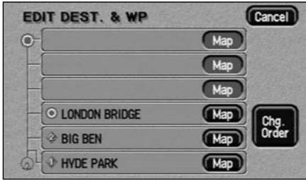
After touching **List**, the list showing the stored way points and destination (if entered) is displayed. The first way point to be visited is at the bottom of the list and the destination at the top.
