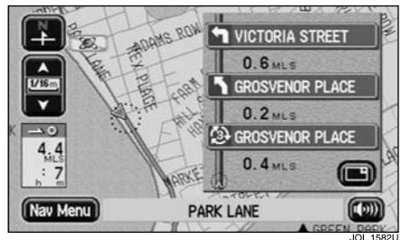
When set to Turn List, the guidance screen overlay shows the current portion of the route turn list. Before each manoeuvre point, the next junction diagram is displayed.
