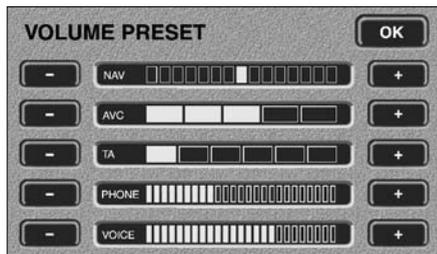
This maintains radio volume at a level sufficient to overcome road noise as vehicle speed increases or decreases. To activate AVC, press the **MENU** button, followed by the **VOLUME PRESET** button on the touch-screen. Once in the volume preset screen, AVC level can be adjusted (from OFF to 5) by repeatedly pressing the '+' or '-' buttons adjacent to the AVC volume indicator.
