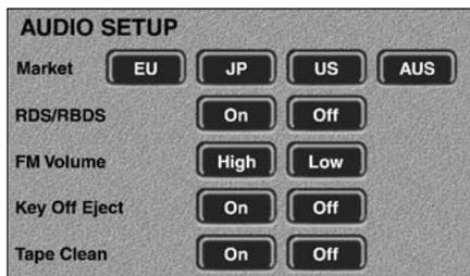
This function enables the radio to be set to user operating preferences. By selecting **SETUP** and using the buttons on the touch-screen, the owner or Jaguar Retailer can adjust certain radio functions. When in **SETUP**, pressing the relevant button will display the facility selected and its state. The state of that facility can be changed by pressing the button again.
