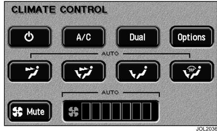
Automatic operation provides a controlled environment over a temperature range of 61°F to 89°F (17°C to 31°C) and should be regarded as the normal operating mode.
