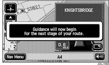
When the vehicle arrives at a way point, the screen shows 'You have arrived at your Way Point'. When the journey is resumed, route guidance continues automatically, either to the next way point or to the final destination.
