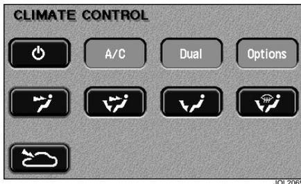
With the climate control system switched off, air recirculation is automatically selected (intake flap closed).
