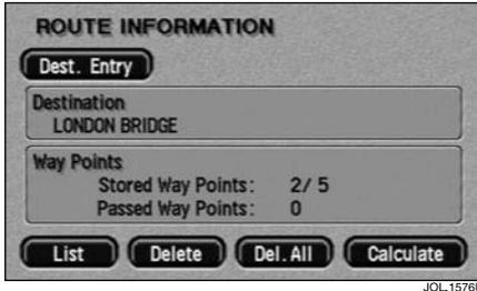
If the destination has been entered, then, after storing the final way point, the route calculation can be started from the Route Information screen. This screen should now show details of the destination, and the number of way points entered.
