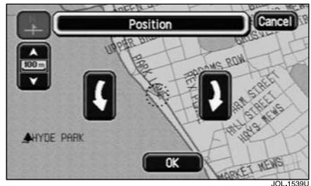
The map screen showing the heading adjustment arrows is displayed.
