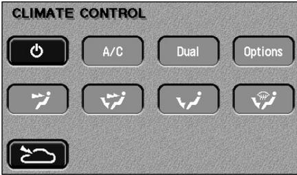
To switch the system off, touch the system ON/OFF button on the CLIMATE CONTROL screen. The touch-screen will change to the system off/ram air climate control screen above.
