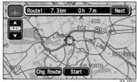
Following calculation, the screen shows the whole route, with the total route distance, and estimated travelling time displayed at the top of the screen. Up to three possible routes are calculated.
