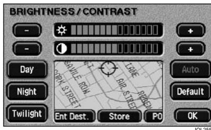
After touching the **Brightness/Contrast** button, the screen displays the buttons for adjustment of the screen display characteristics. The centre window shows the currently selected navigation view.
