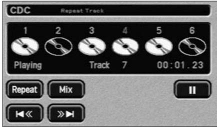
In CD changer mode, touch-screen buttons (shown above) provide for track and disc selection. Discs present in the magazine are highlighted in the display.
